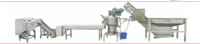
The PL peelers are ideally suited to be integrated in complete and continuous root processing lines for washing, peeling, cutting / dicing up to 1.200 kg per hour. The loading and peeling process is central controlled.
