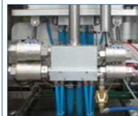
DOUBLE VALVE VACUUM & GAS SYSTEM / DOPPELTES VAKUUM & GAS VENTIL SYSTEM
