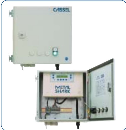
W380 option for SHARK controller SHARK digital control box for rough industrial environment, wall installation. 3 m sensor link cable, power supply 85–264V/50–60Hz. Housing size 380 x 380 x 210 mm. Available for METAL SHARK® TU, FL, GF, GFC,R.
