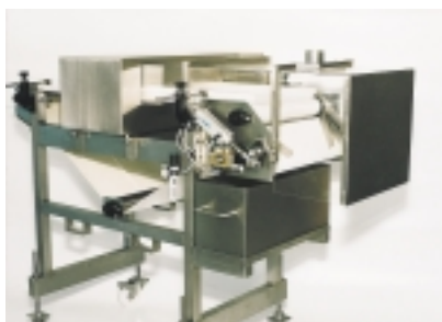
Reject option: Switching flap at belt end
