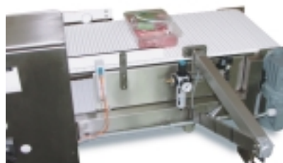
Reject option: Pneumatic transversal pusher (for packed foods)
