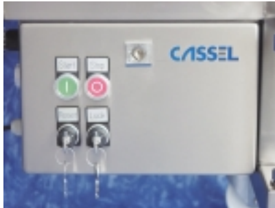
Belt control unit, with optional turn key buttons (lock keyboard, reset metal alarm)
