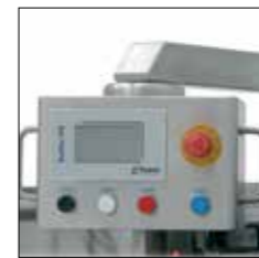
MULTIFUNCTIONAL DISPLAY WITH TOUCH SCREEN PAD ON MOVABLE ARM / MULTIFUNKTIONSDISPLAY (TOUCH SCREEN, SCHWENKBAR)
