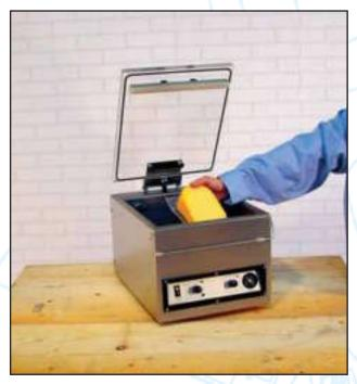
The Mini-jumbo is a vacuum sealer with a vacuum chamber of 280x 350x 80mm. The seal time and vacuum time on this machine can be individually adjusted. The Mini-Jumbo allows you to quickly and easily produce vacuum packed articles.
