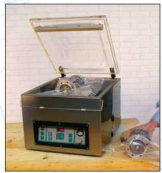
The VAC-200-XL is a vacuum sealer with a vacuum chamber of 420x 370x 170mm. This machine is equipped with 10 programs, allowing you to quickly vacuum pack different types of products, one after another, without the need to readjust the settings on the machine.
